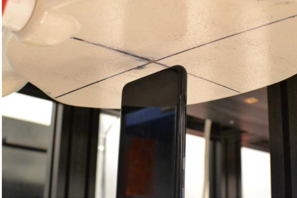
SAR Test Setup Photo 13 – Bottom Side at 10 mm
