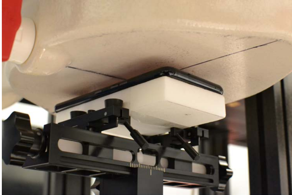
SAR Test Setup Photo 5 – Back Side at 10 mm
