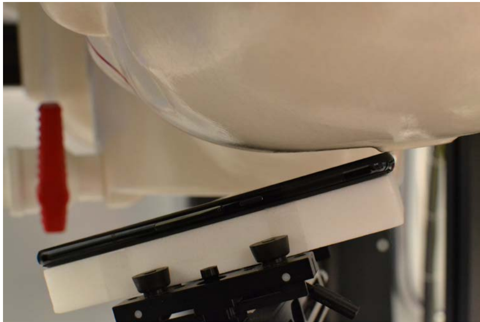
SAR Test Setup Photo 4 – Left Tilt
