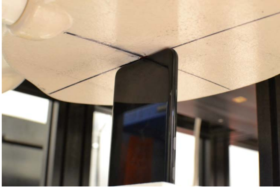
SAR Test Setup Photo 15 – Bottom Side at 0 mm
