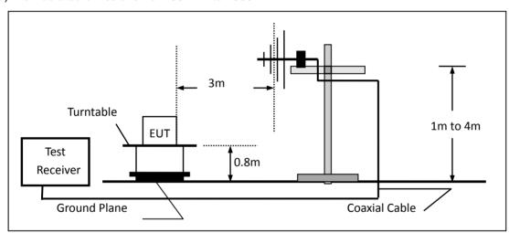
(c) For radiated emissions above 1000MHz
