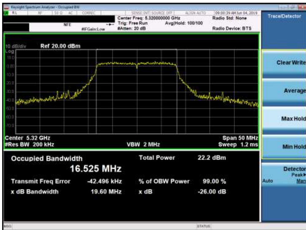
Plot 7-12. 26dB Bandwidth Plot (802.11a (UNII Band 2A) – Ch. 64)
