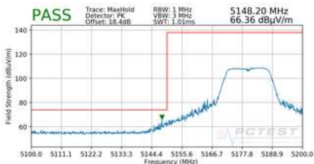
Plot 7-84. Radiated Lower Band Edge Plot (Peak – UNII Band 1)
