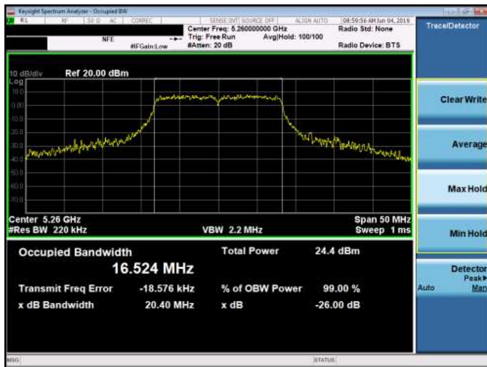
Plot 7-10. 26dB Bandwidth Plot (802.11a (UNII Band 2A) – Ch. 52)
