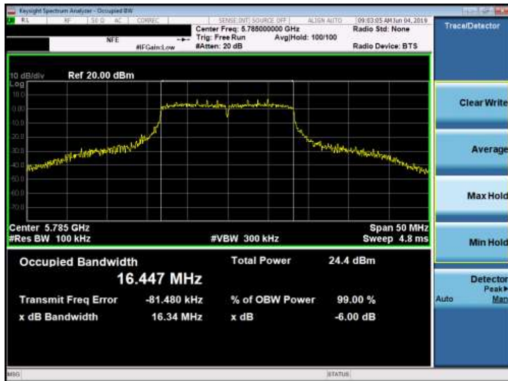
Plot 7-31. 6dB Bandwidth Plot (802.11a (UNII Band 3) – Ch. 157)
