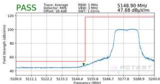
Plot 7-83. Radiated Lower Band Edge Plot (Average – UNII Band 1)
