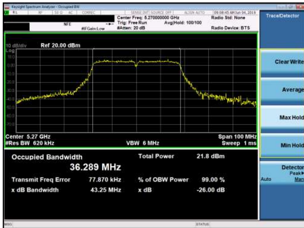
Plot 7-16. 26dB Bandwidth Plot (40MHz BW 802.11n (UNII Band 2A) – Ch. 54)
