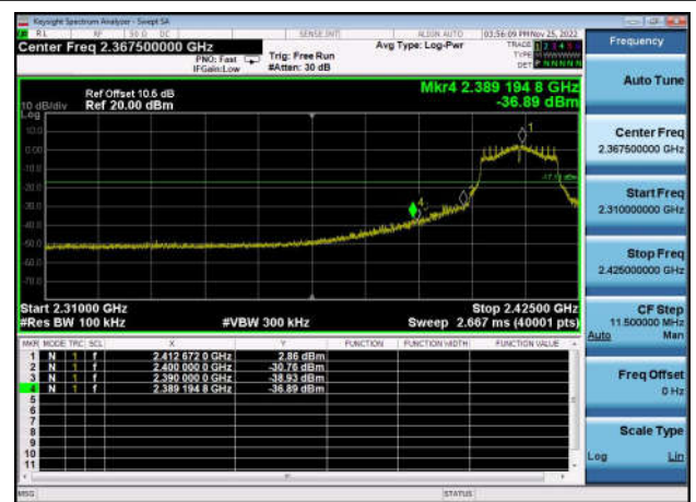
,Plot 2,Band Edge-802.11g,2462MHz ,Ant0
