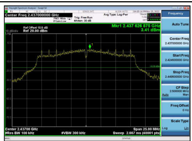
,Plot 2,Band Edge-802.11g,2412MHz ,Ant0
