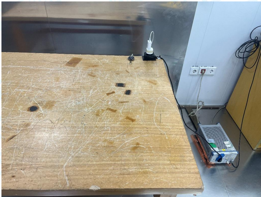
Photo of Setup for Conducted Emission
