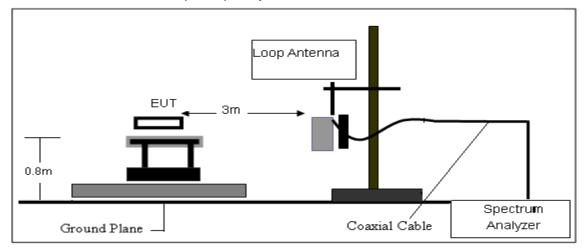
(B) Radiated Emission Test-Up Frequency 30MHz~1GHz
