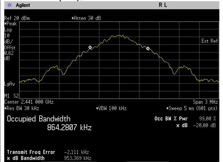
ii. The 20 dB BW & occupied bandwidth test with result at mid frequency, GFSK.
