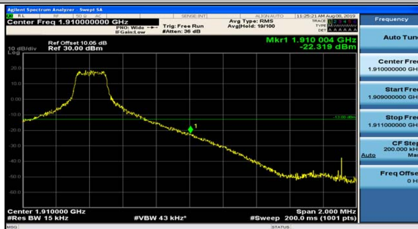
Channel Bandwidth: 10 MHz_HCH_16QAM_25RB#0
