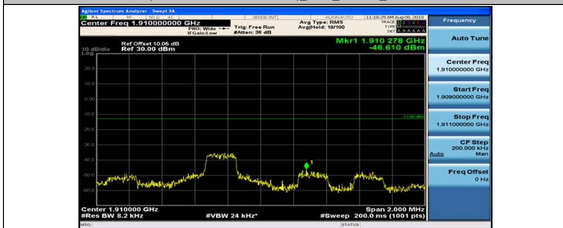
(Channel Bandwidth: 3 MHz)_HCH_16QAM_1RB#7
