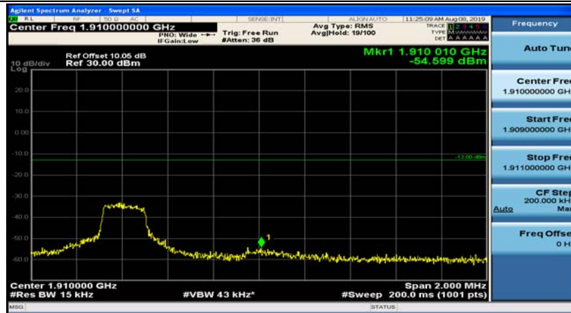
Channel Bandwidth: 10 MHz_HCH_16QAM_1RB#24
