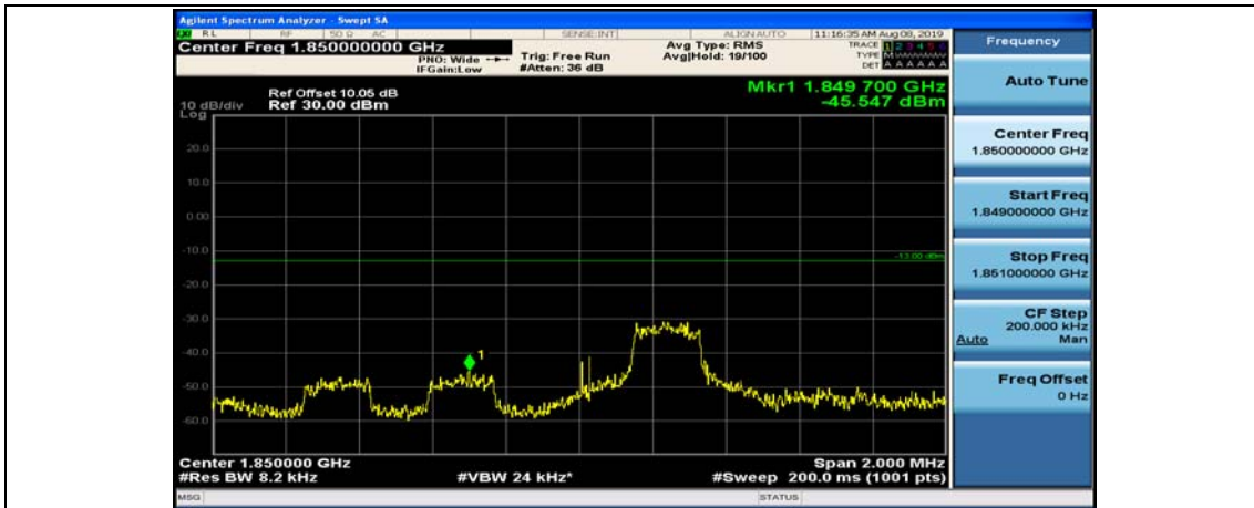
(Channel Bandwidth: 3 MHz)_LCH_QPSK_8RB#0
