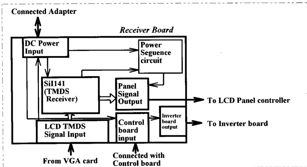
The most important job of the receiver board is to receive TMDS signals transmitted from the TMDS transmitter IC, SiI140, on the VGA card and to transfer these signals to CMOS/TTL level signals and send to LCD panel controllers. As following the specification of the LCD power sequence to protect LCD panel from DC charge and damaged.
