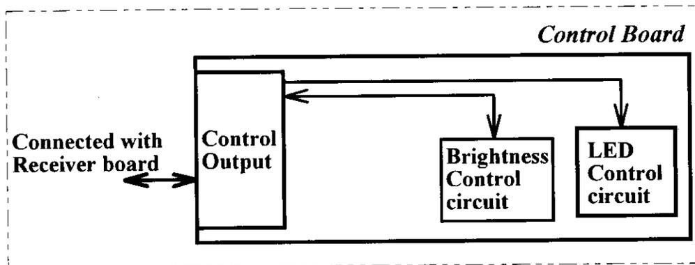
The jobs of the control board are to output brightness control voltage to the inverter board and to drive the LED to display the LCD monitor operating status.
