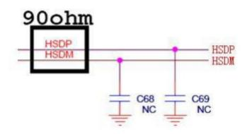
Note: USB D + / D-differential line impedance control 90 OHM; C 68 and C 69 should be reserved in advance and adjusted according to the actual situation;
