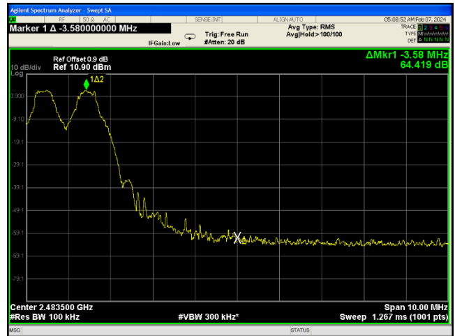
Band Edge - High Channel Hopping Enabled Center Freq. 2.4835GHz
