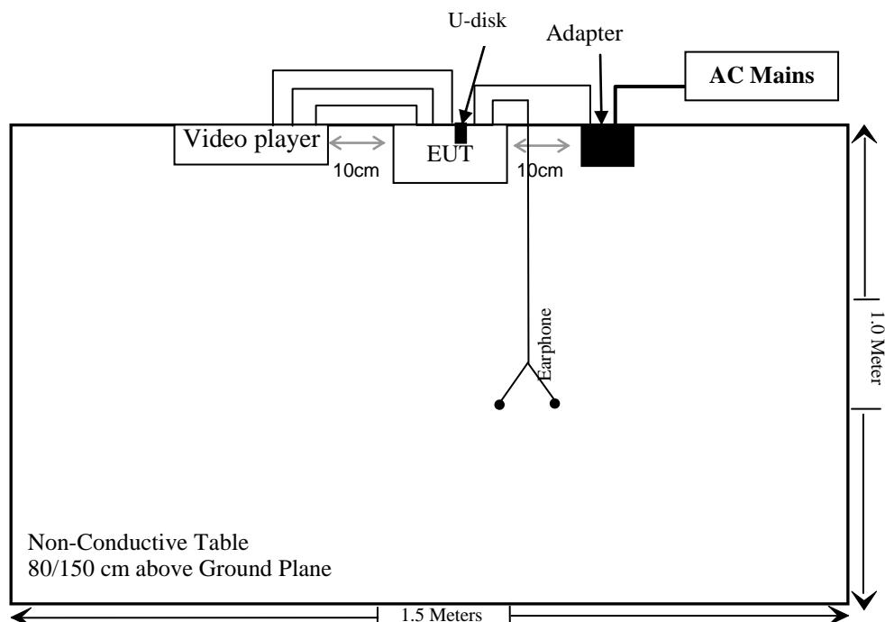
Note: the support table edge was flush with center of turntable
