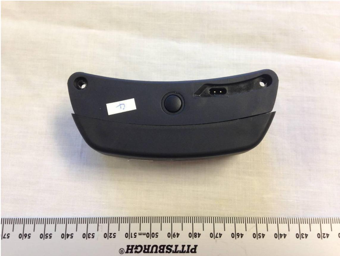
**Figure 2. EUT w/ Collar and Antenna Removed**
