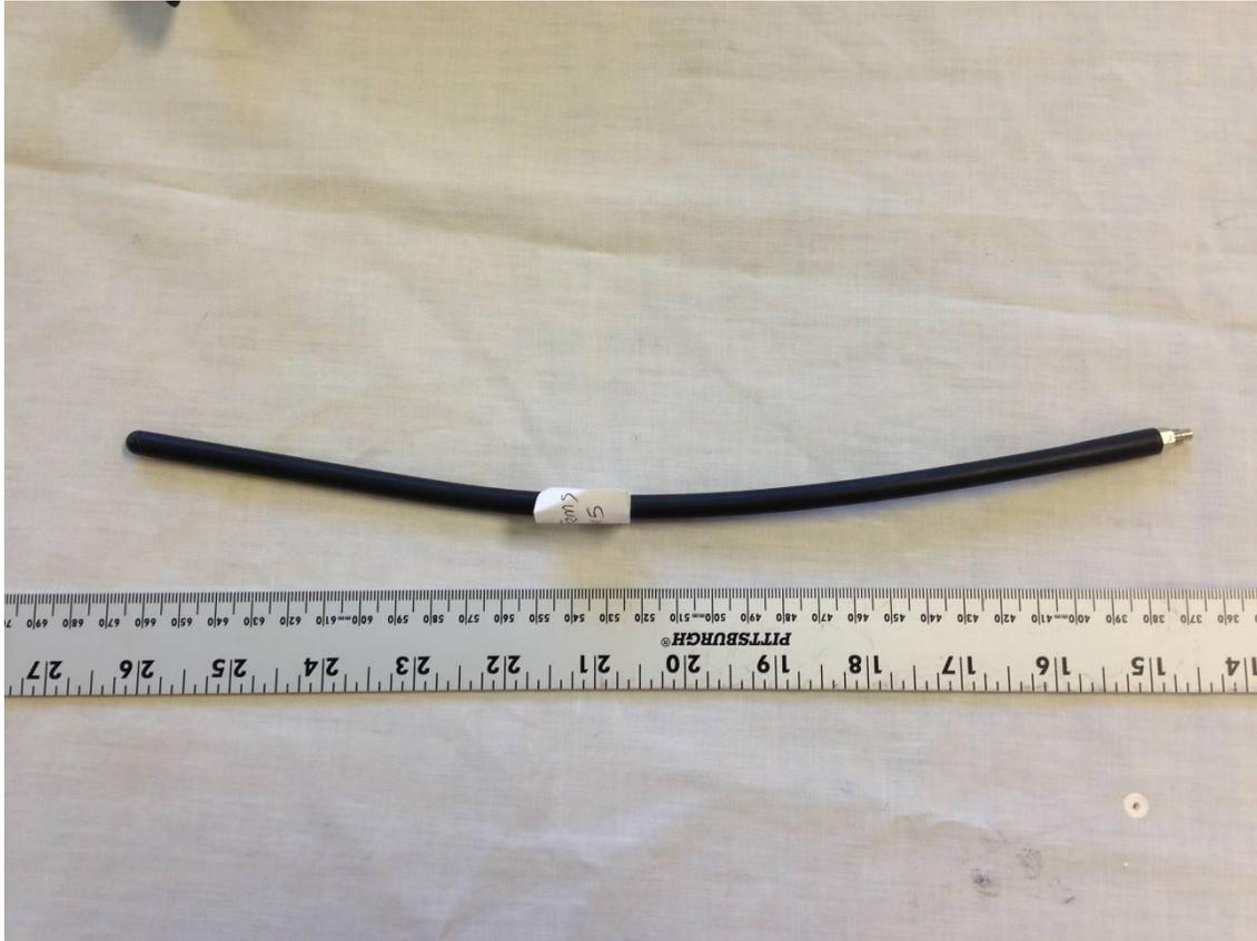
**Figure 7. EUT Antenna**
