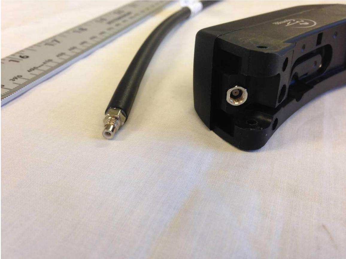
**Figure 8. EUT, Unique Antenna Connector**
