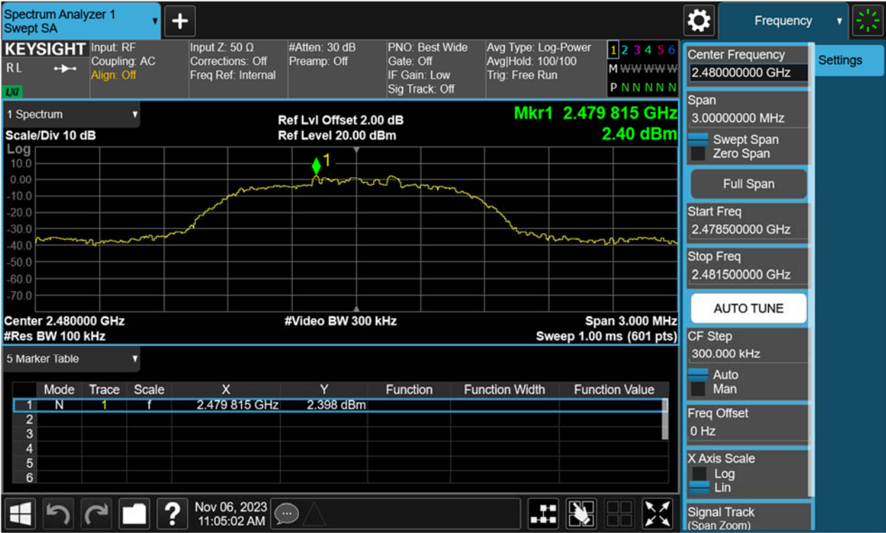
Figure 24: Conducted Spurious Emission & Authorized-band band-edge, 2480MHz, \pi/4 -DQPSK Carrier Level
