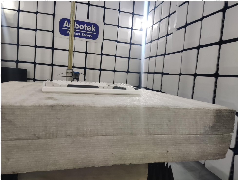
Photo of Radiation Emission Test (above 1GHz)
