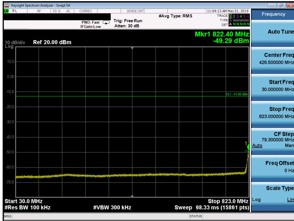
Plot 7-54. Conducted Spurious Plot (Band 5 - 10.0MHz QPSK - RB Size 1, RB Offset 0 - Low Channel)
