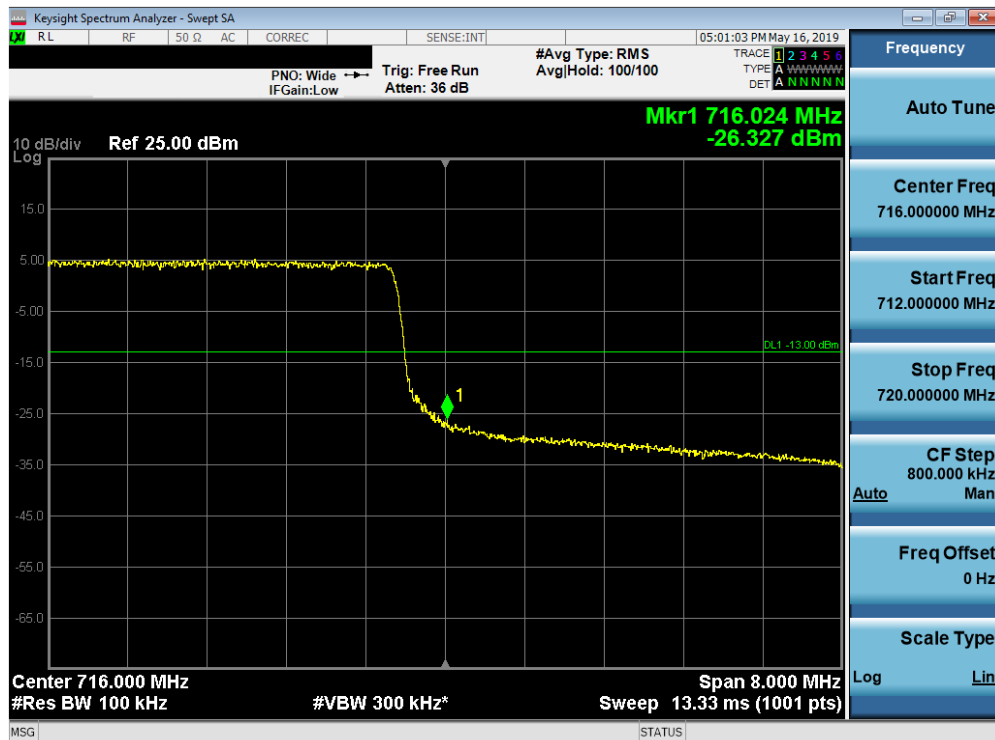
Plot 7-91. Upper Band Edge Plot (Band 12 - 10.0MHz QPSK - Full RB Configuration)
