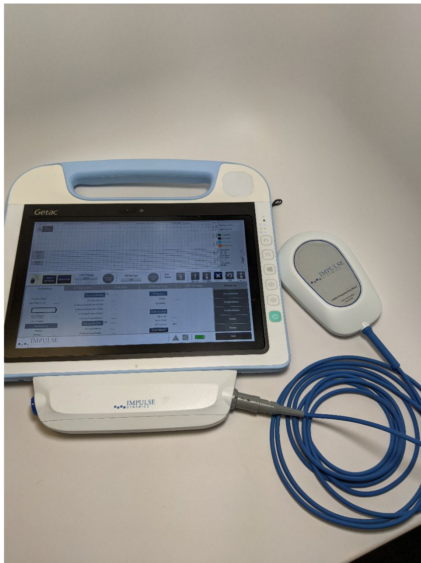
External Picture 3: Picture of Intelio Programming Wand in intended use, attached to external Intelio Programming Interface and tablet.
