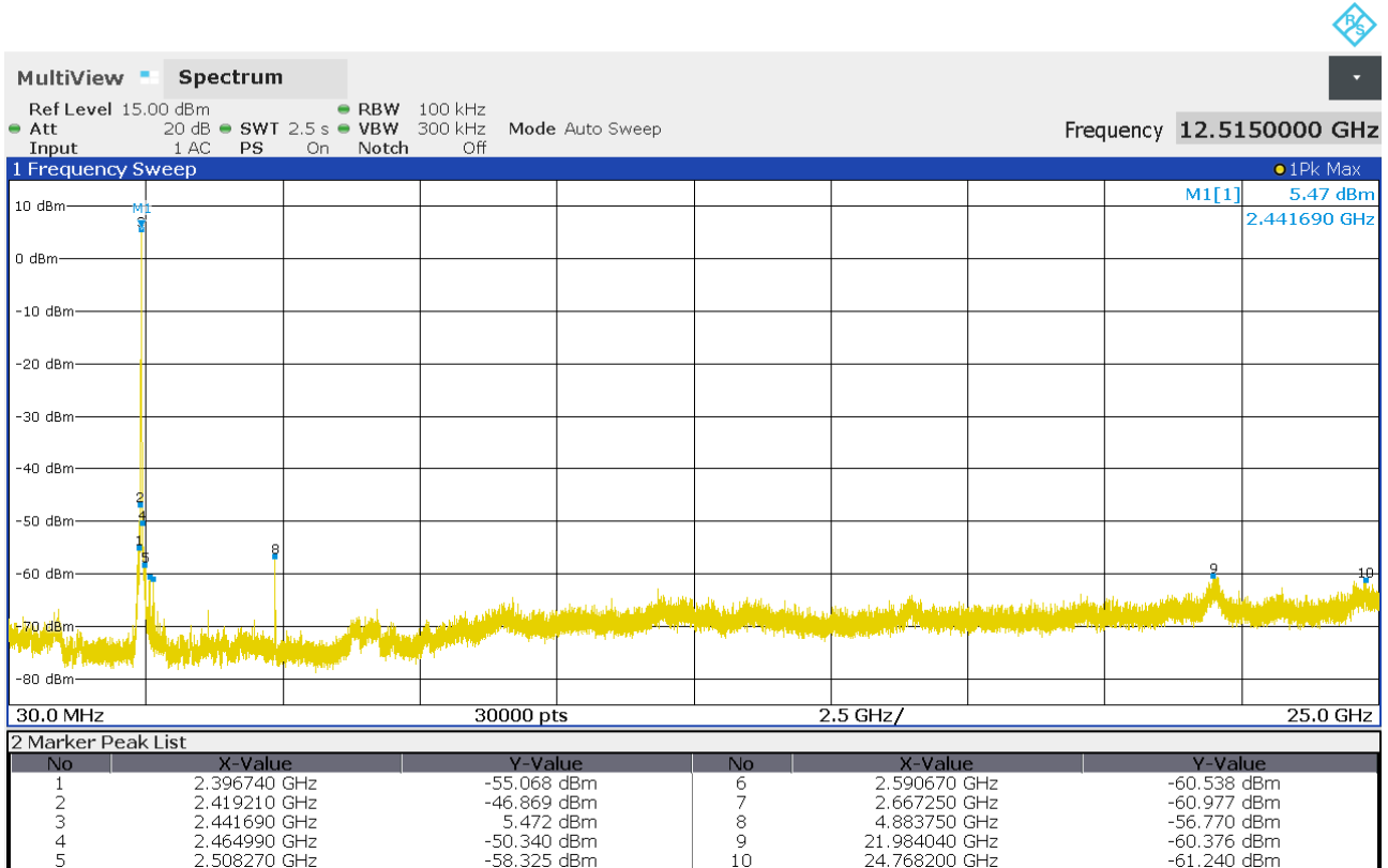
Figure 33 Conducted emissions 30MHz to 25GHz. Operation on IEEE 802.11b channel 2442MHz.
