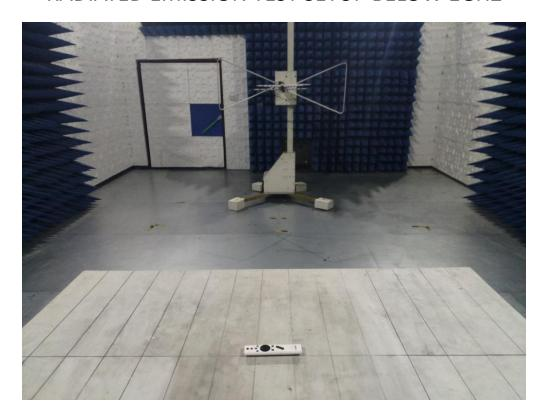
RADIATED EMISSION TEST SETUP ABOVE 1GHZ
