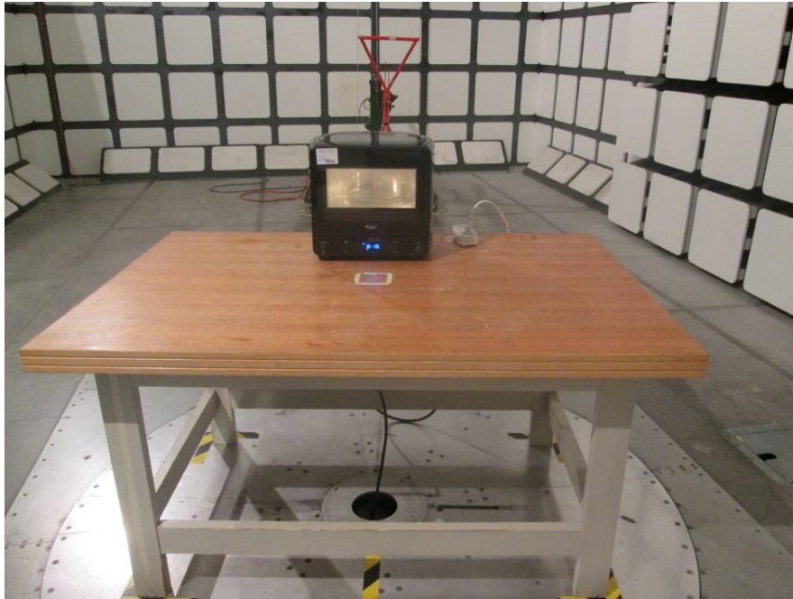
Radiated Emissions - Front View (30 MHz – 1 GHz)
