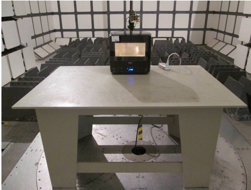
Radiated Emissions - Front View (Above 1 GHz)
