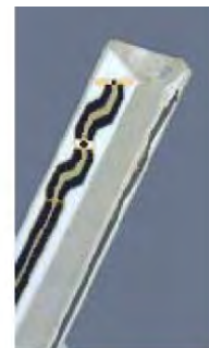
Figure 3.3 Probe Thick-Film Technique
