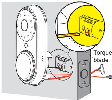
**C** Secure the mounting plate with the supplied screws. Short Mounting plate screws are applied to the door with thickness of 35mm-45mm. Long Mounting screws are applied to the door with thickness of 45mm-50mm. Do not overtighten screws.
