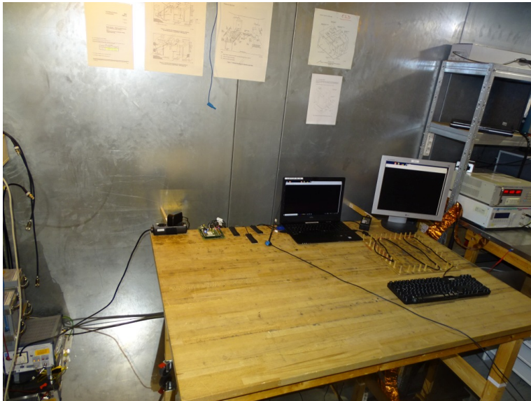
Photo 3: Test setup for conducted measurement
