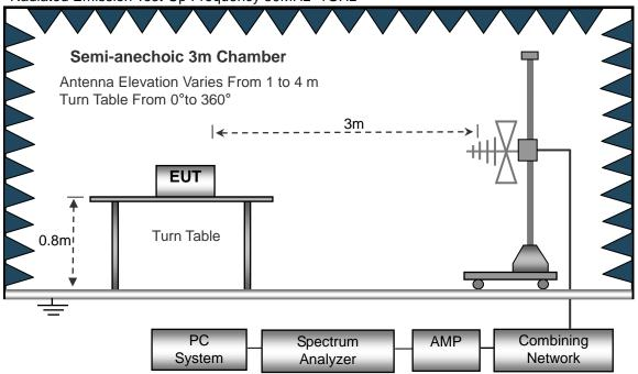
(C) Radiated Emission Test-Up Frequency Above 1GHz
