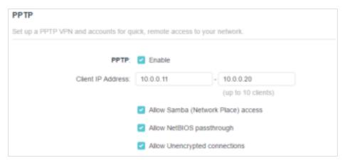
Note: Before you enable VPN Server, we recommend you configure Dynamic DNS Service (recommended) or assign a static IP address for router's WAN port and synchronize your System Time with internet.
