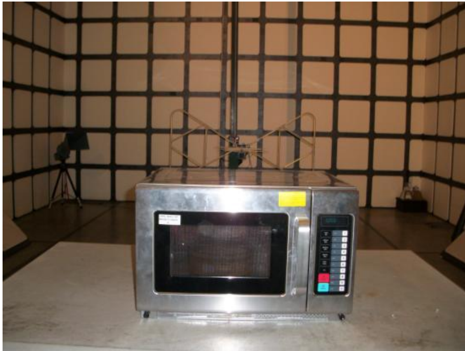
Radiated Emission Test Set-up (30 -1,000MHz)
