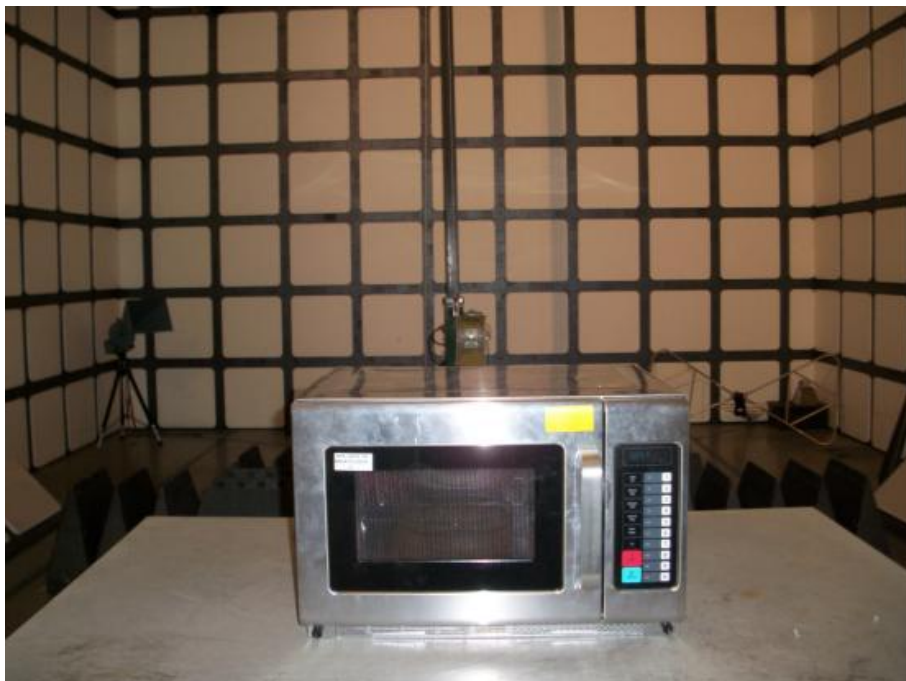
Radiated Emission Test Set-up (1-18GHz)
