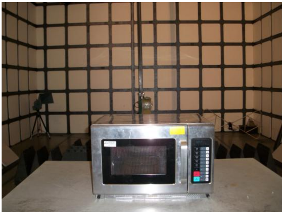
Operating Frequency Test Set-up
