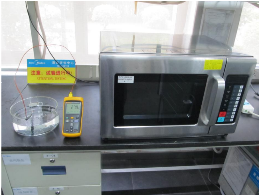
RF Output Power Test Set-Up
