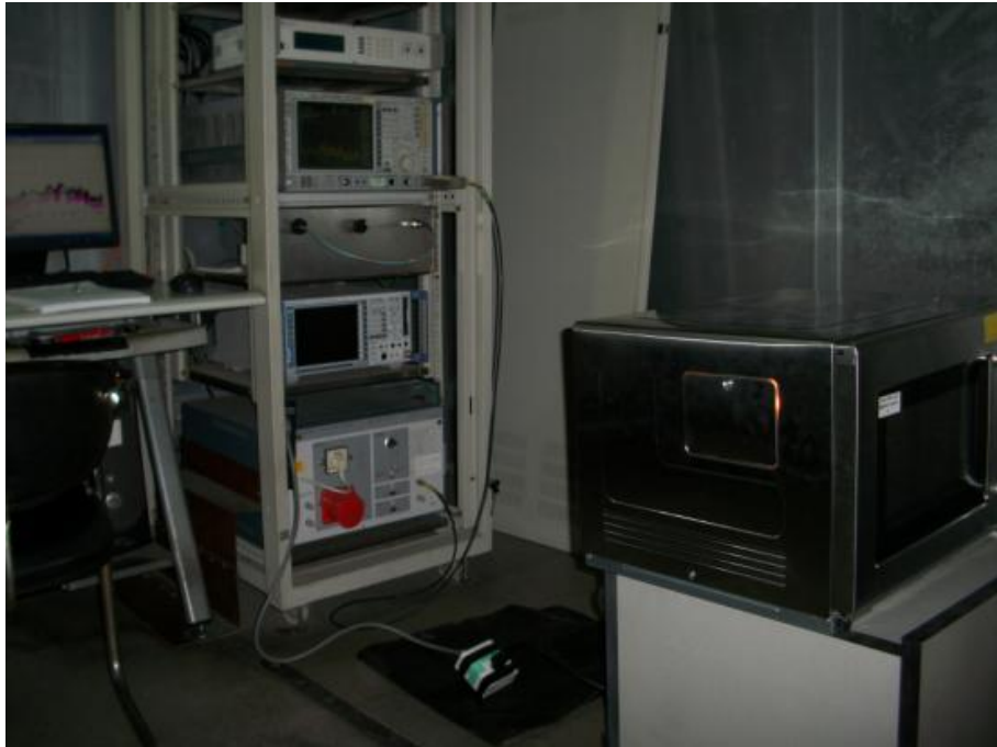
Conducted Emission Test Set-up
