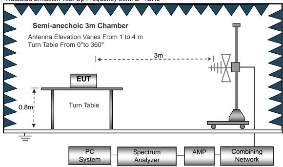
(C) Radiated Emission Test-Up Frequency Above 1GHz
