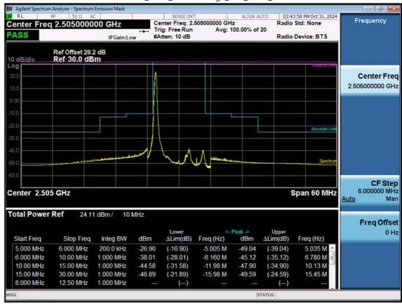
LTE B7\_10 M\_Channel Edge\_Low\_QPSK\_1RB
