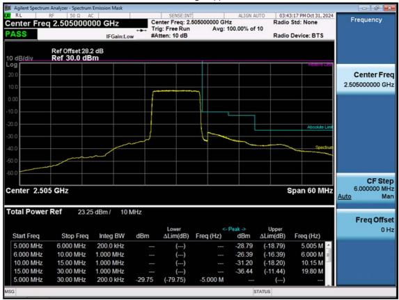
LTE B7\_10 M\_Channel Edge\_Upper\_Low\_QPSK\_FullRB
