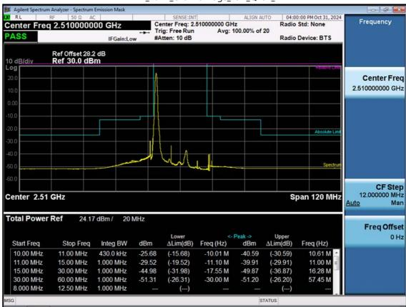
LTE B7\_20 M\_Channel Edge\_Low\_QPSK\_1RB
