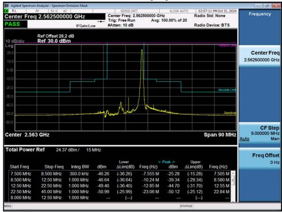
LTE B7\_15 M\_Channel Edge\_High\_QPSK\_1RB
