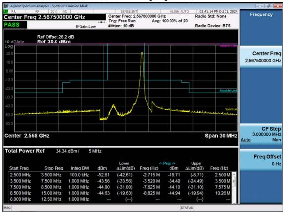
LTE B7\_5 M\_Channel Edge\_High\_QPSK\_1RB
