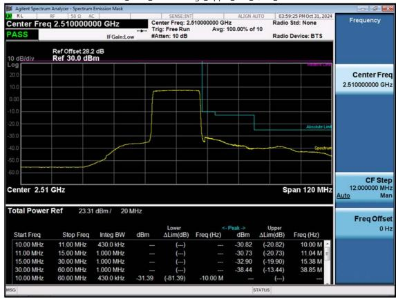
LTE B7\_20 M\_Channel Edge\_Upper\_Low\_QPSK\_FullRB
