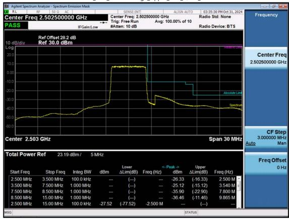
LTE B7\_5 M\_Channel Edge\_Upper\_Low\_QPSK\_FullRB
