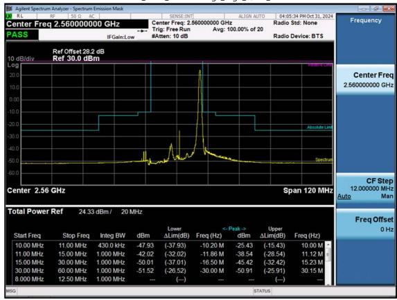
LTE B7\_20 M\_Channel Edge\_High\_QPSK\_1RB
