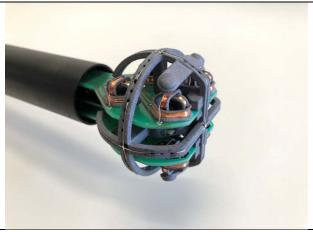
Test probe, without the casing
