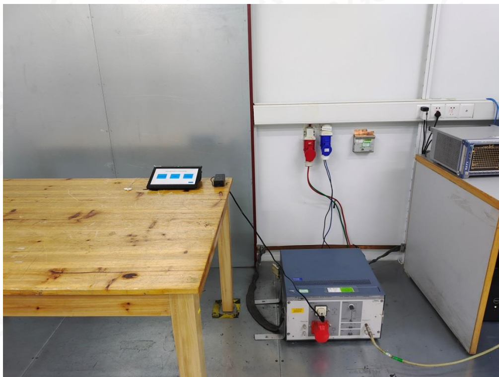
RADIATED EMISSION TEST SETUP BELOW 1GHZ
