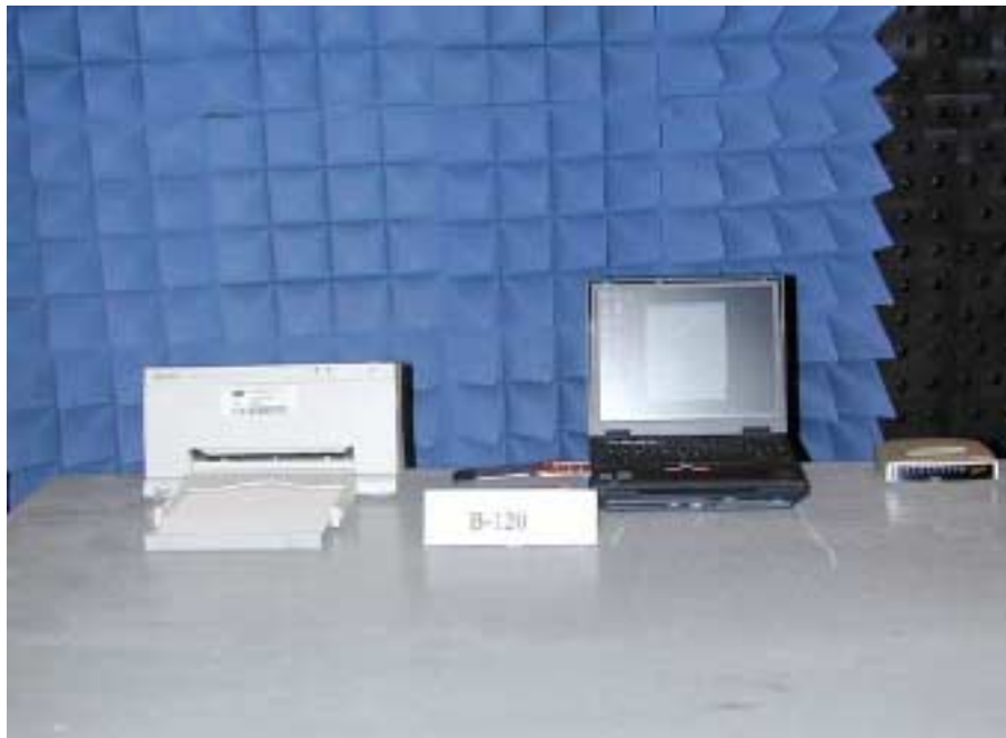
Photo 1: Spurious Test Set-up (front)
