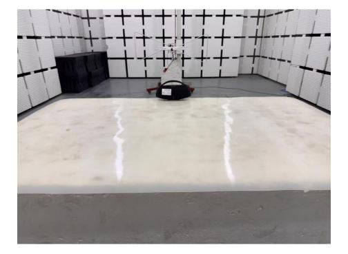
Set-up for Radiated Spurious Emission, Below 1GHz
