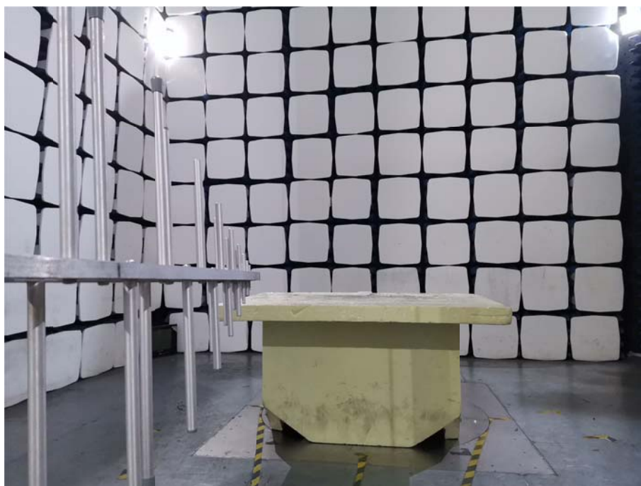
Radiation Emission Test Setup (30MHz to 1GHz)
