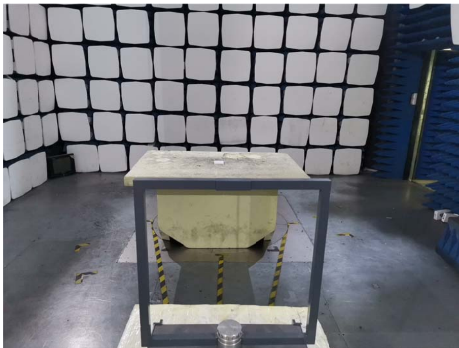
Radiation Emission Test Setup (Below 30MHz)
