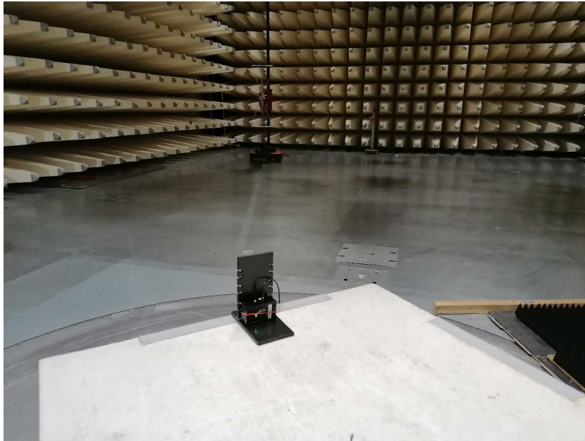
Photo 1: EUT at the semi-anechoic chamber
