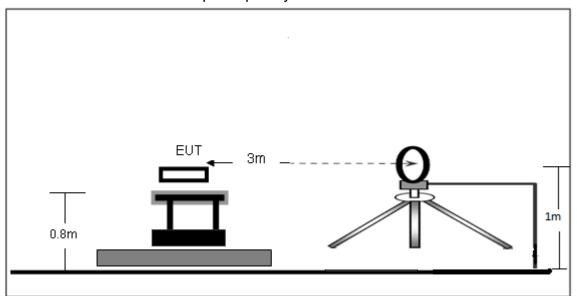
(B) Radiated Emission Test-Up Frequency 30MHz~1GHz
