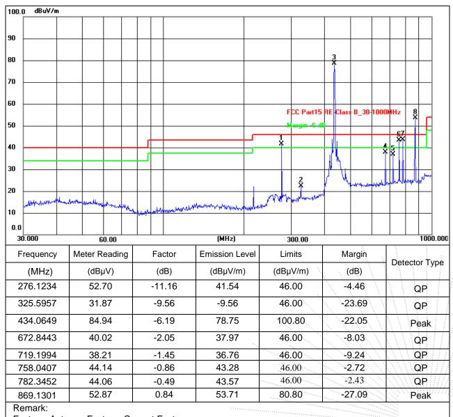
Factor = Antenna Factor + Correct Factor. Correct Factor= Cable Loss - Pre-amplifier
