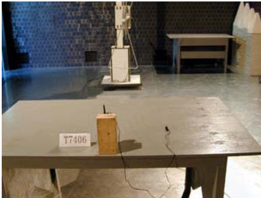
Photo 5: Spurious emission setup (Handset unit)
