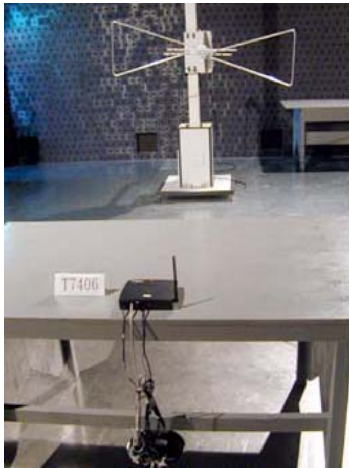
Photo 1: Spurious emission setup (Base unit)
