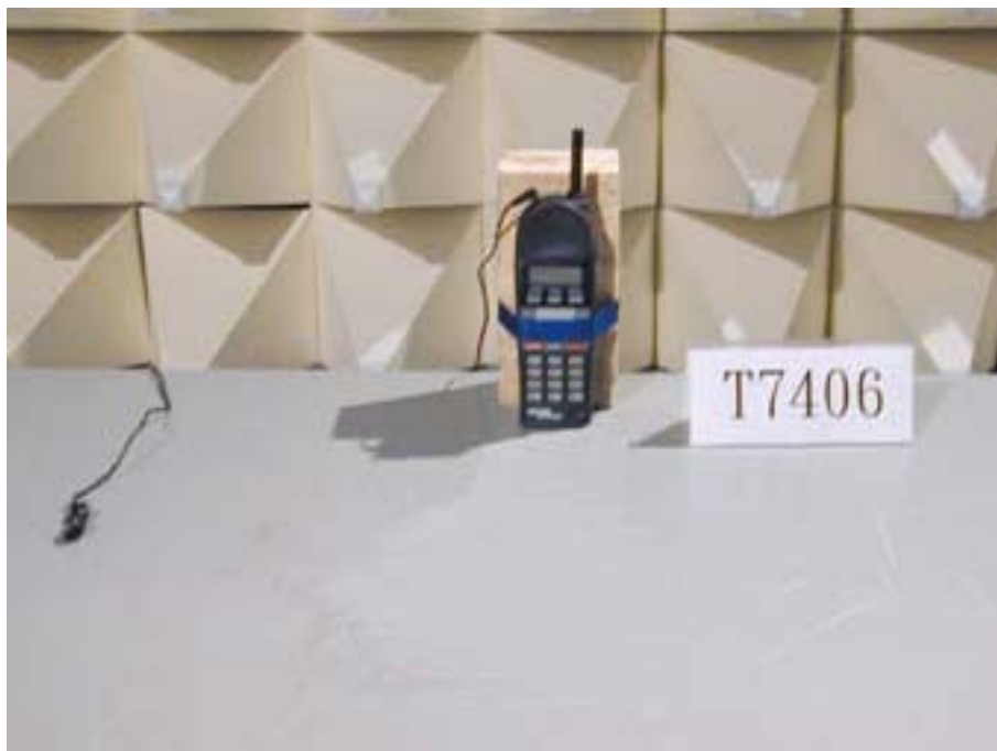
Photo 6: Spurious emission setup (Handset unit)
