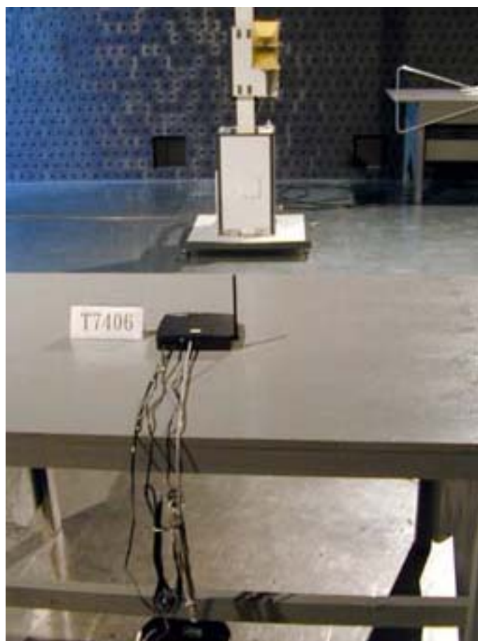
Photo 3: Spurious emission setup (Base unit)
