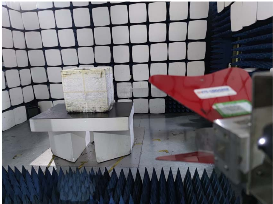
Radiation Emission Test Setup (1GHz to 18GHz)
