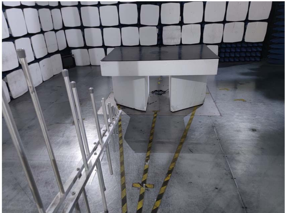
Radiation Emission Test Setup (30MHz to 1GHz)
