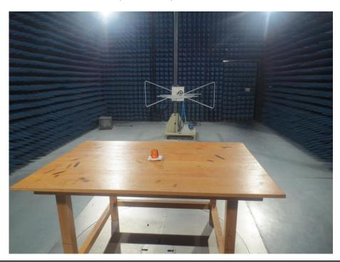
Description: Radiated Emission Test(Above 1 GHz)
