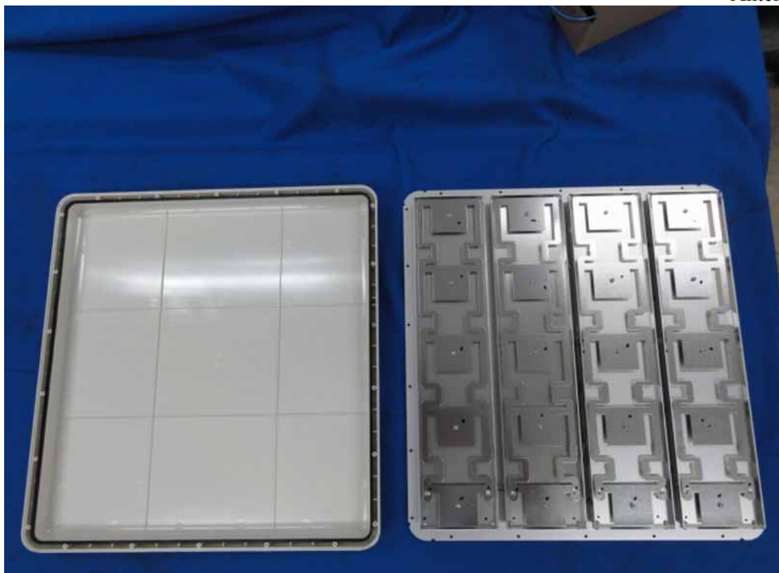
Figure 39 Antenna for 2.4G
