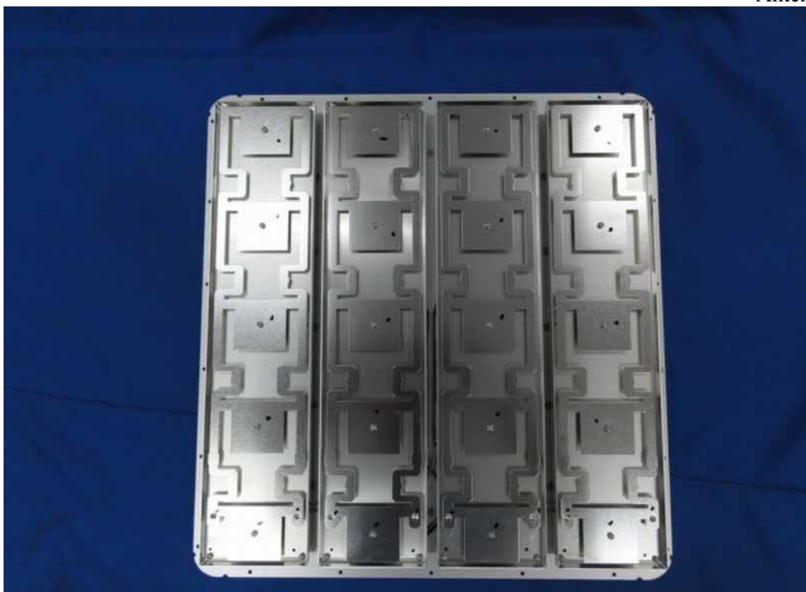
Figure 40 Antenna for 2.4G
