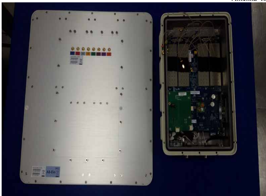
Figure 37 Antenna for 2.4G
