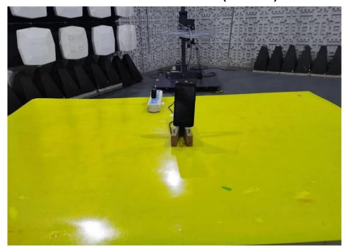
1.8 Unwanted Emissions that fall Outside of the Restricted Bands(Radiated) and Unwanted Emissions in the Restricted Bands (Radiated) above 1GHz
