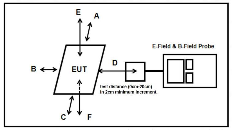
Note: Measurements should be made from all sides and the top of the primary/client pair, the test distance of A, B, C, D, E, F side is 0cm to 20cm.
