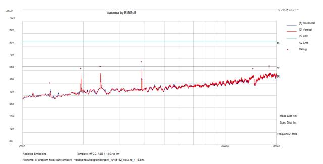
S.A. Correction Corrected Antenna **Antenna Turntable Frequency** Limit Margin Reading **Factor** Amplitude **Azimuth** Height **Polarity Detector** (MHz)  $(dB\mu V/m)$ (dB) (dBuV) (dB/m)  $(dB\mu V/m)$ (cm) (H/V)(degrees) 3890 63.71 -1.77 61.94 200 Η 0 63.54 -1.6 Peak 16640 46.71 11.57 58.28 100 Η 0 63.54 -5.27 Peak
