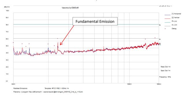
Correction Antenna Corrected Antenna **Turntable** S.A. **Frequency** Limit Margin Reading **Factor** Amplitude Height **Polarity Azimuth Detector** (MHz)  $(dB\mu V/m)$ (dB) (dBuV) (dB/m)  $(dB\mu V/m)$ (degrees) (cm) (H/V)46.98 16714.38 12.02 59 300 V 360 63.54 -4.54 Peak 100 13803.13 45.05 12.06 57.11 Η 360 63.54 -6.43 Peak
