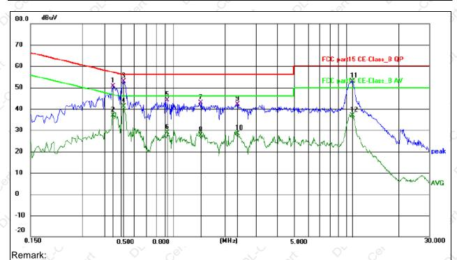
Margin = Limit – Level, Correct Factor = Cable lose + LISN insertion loss, Level= Reading + Correct factor
