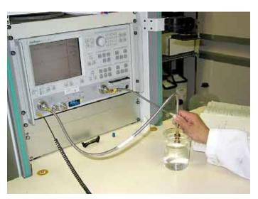
Tissue used during the SAR assessment is calibrated prior to measurement the process. APREL Laboratories use the co-axial probe method for all tissue calibration exercises. Tissue which is being used over a period of 24 hours is recalibrated to ensure that no change to the dielectric properties will affect the SAR measurement process. The table below provides details of the results from the tissue equivalent dielectric calibration.
