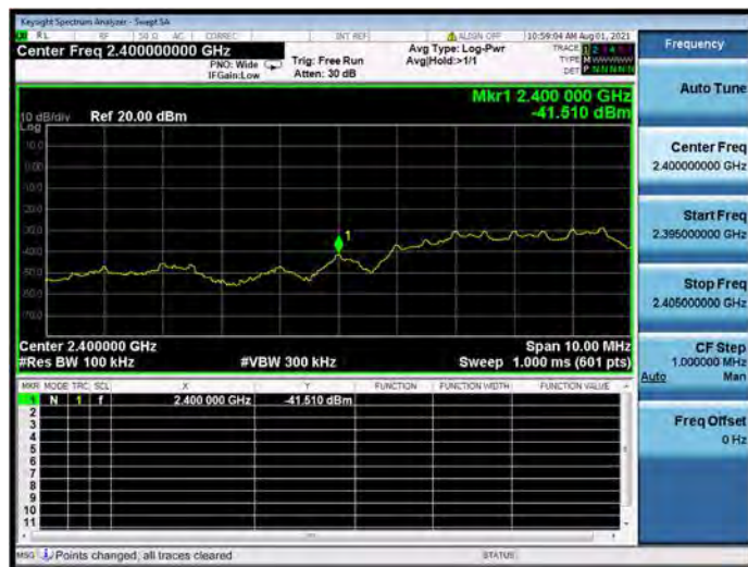
802.11b CHANNEL 2, Carrier level
