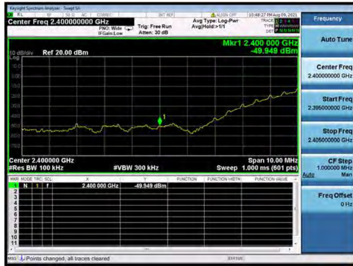
802.11b CHANNEL 1, Carrier level
