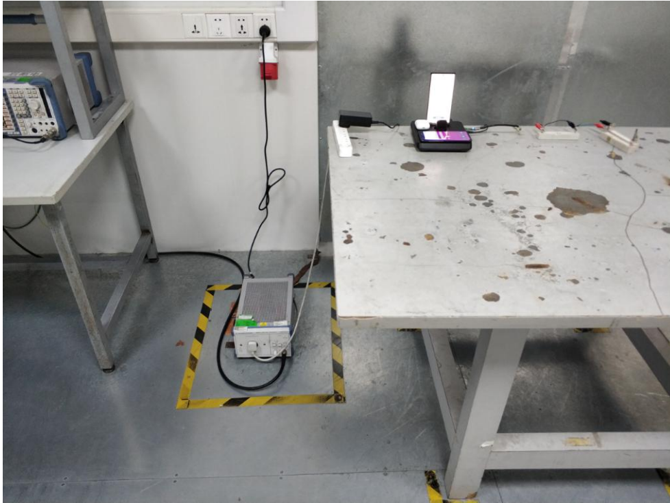
Photo of Conducted Emission Measurement
