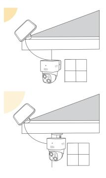
1. Drill holes with a 15/64 inch (5.95 mm) drill bit with the provided positioning card, then insert the anchors into the holes.
