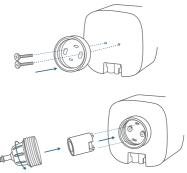
2. Install the solar panel onto the solar panel's mounting bracket by turning it.
