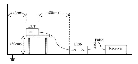
(For Conducted Emission, AC Ports Test)
