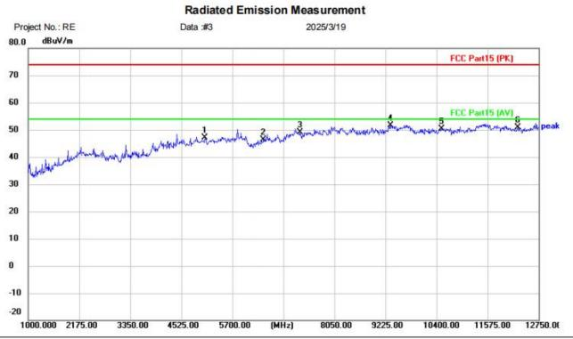
Site Polarization: Horizontal Temperature: (C)
