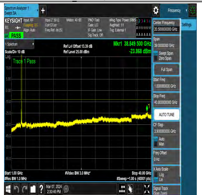
NTNV-N77-3700-3980-PC2-30-100-M-DFT-QPSK-Edge_1R B Left-Ant5-PASS
